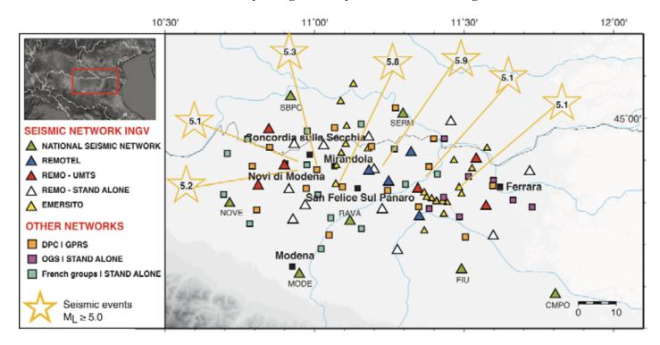
**Figure 3.** Map of the seismic stations deployed after May 20, 2012. Triangles, INGV permanent (green) and temporary stations; squares, stations from other Institutes; stars, earthquakes with magnitude >5.0.
